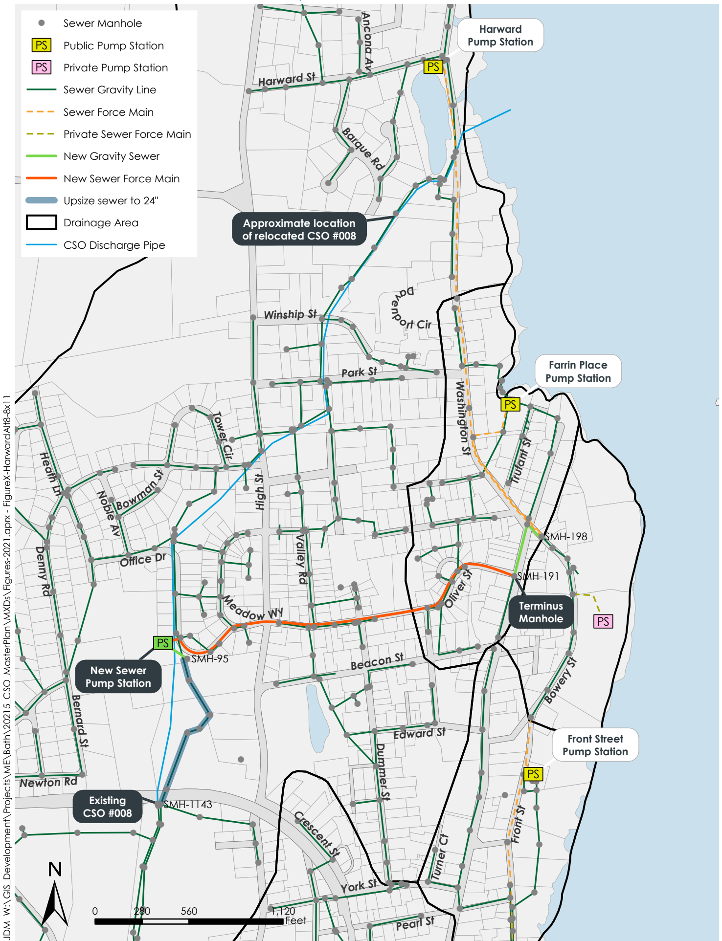
Figure E-11 Harward Street CSO: Alternative 8 – Collection System Capacity Increases (Alt 2, Phase 1, and Phase 3), New Sewer Pump Station (Alt 3), and Relocate CSO #008 (Alt 4)
