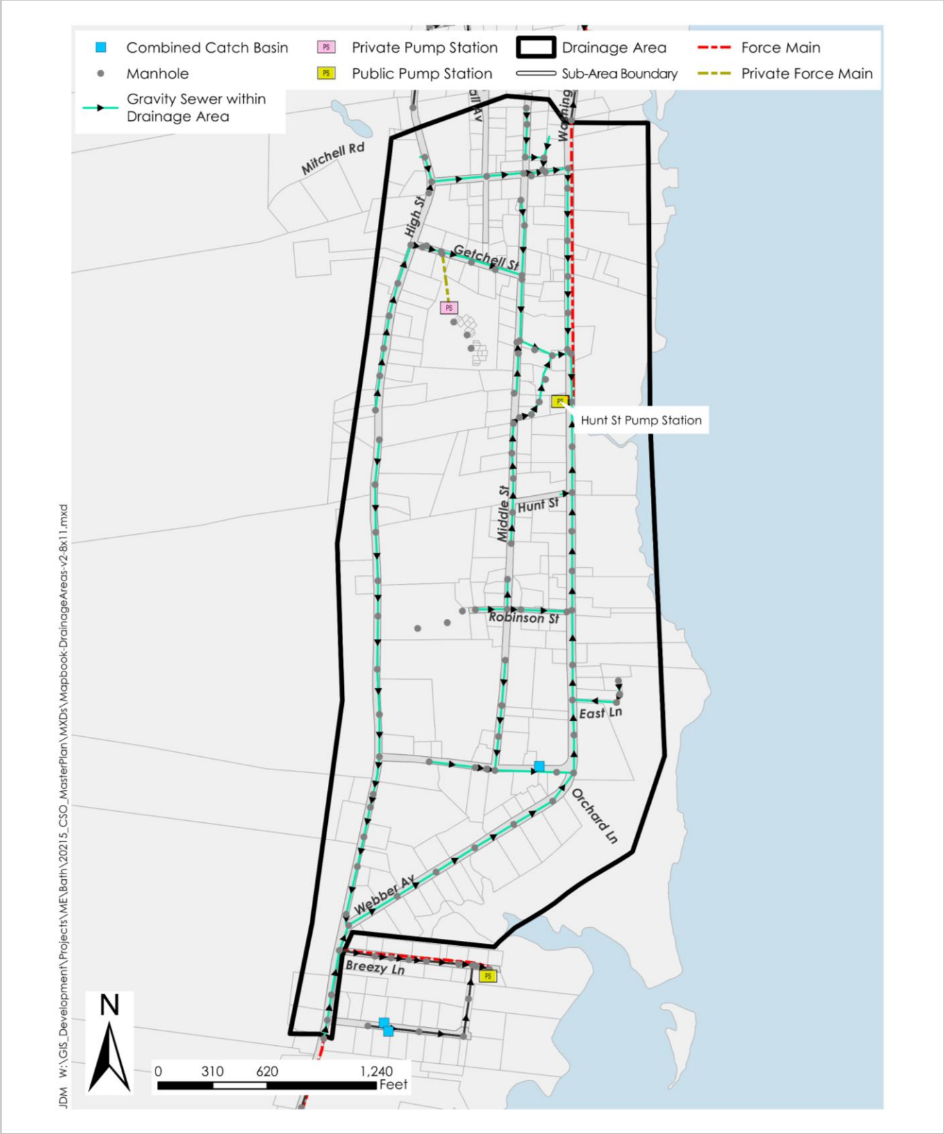
Figure 5-7 Hunt Street Pump Station Drainage Area
