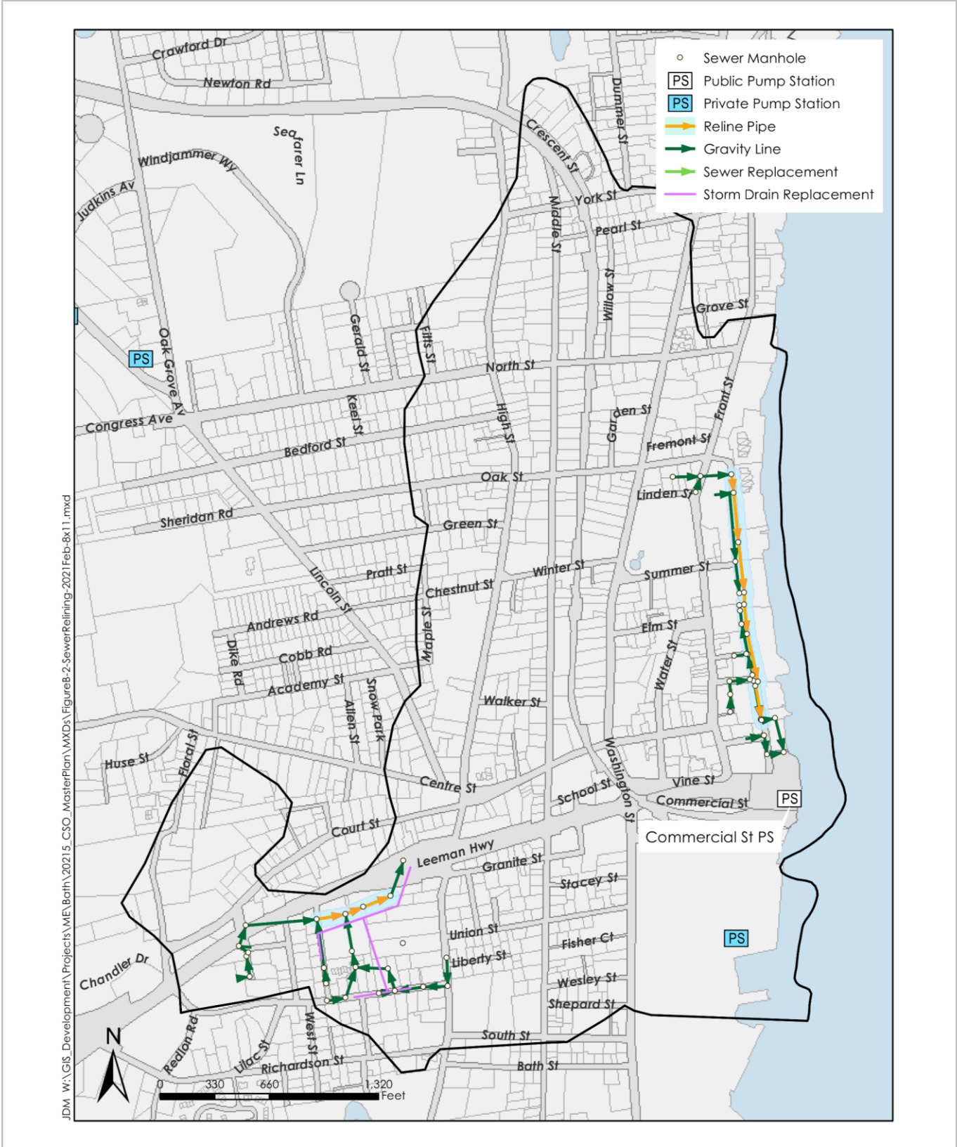
Figure 5-13 Western Ave, Academy Street and Cobb Road Storm Drain and Sewer Improvements Project
