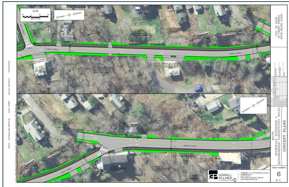
Bike lanes will be striped along the corridor. This includes additional intersection striping and a proposed transition from a separated bike lane to a shared lane at the intersection of Front Street and Holly Street. This transition occurs since Front Street changes from a southbound one-way street south of Holly Street to a northbound one-way street north of Holly Street.
