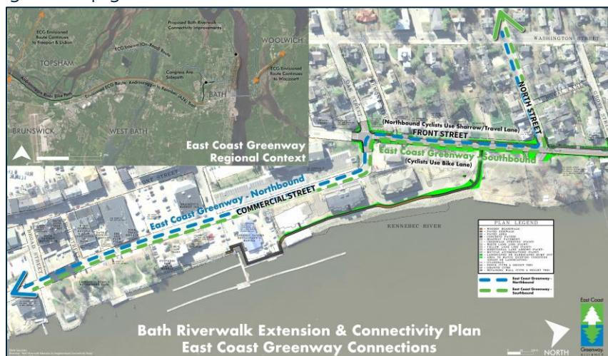
Bike lanes will be striped along the corridor. This includes additional intersection striping and a proposed transition from a separated bike lane to a shared lane at the intersection of Front Street and Holly Street. This transition occurs since Front Street changes from a southbound one-way street south of Holly Street to a northbound one-way street north of Holly Street.
